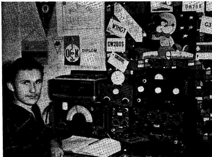
Dvoracek Jaroslav, OL4AFI, Valtirov 97, Usti N. Labem, Czechoslovakia, has made himself very well known on 160 metres. He is a consistent signal all over the U.K. and has worked stations in all parts of the country, including GI and GM. He runs a simple three-stage VFO EF80-buffer EF80-EL36 PA, and his Rx is no more than a modified R.1155. The aerial is, of course, the answer—it is an inverted-Vee, with about 120ft. in each leg. OL4AFI wants us to say, for him, that he is struggling with English, but is learning, and that he is very grateful for the excellent QSL return—he now has about 150 G cards. We gather that Dvoracek is bobbing on his full OKI licence—we would not think that there could be any difficulty about that. Incidentally, there may be some old timers who would remember the famous OK3SI, of the early 1930's, who used to be a consistent evening signal on 160m. running only 3 watts. OL4AFI is in the same tradition.
